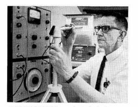
HIGH FREQUENCY sounds study, being conducted by C. P. Skillern (3311), includes measurement on sound level meter of cycles emitted by a small ultrasonic cleaner. The sensitive microphone can record up to 200,000 cycles per second.
